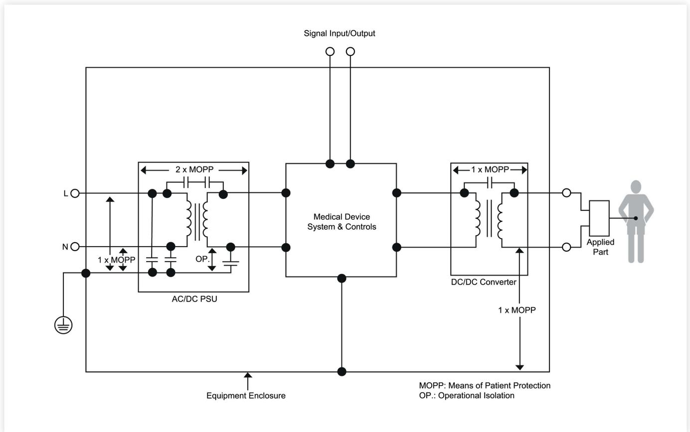
Figure 1: Medical power system with secondary DC/DC isolation.
