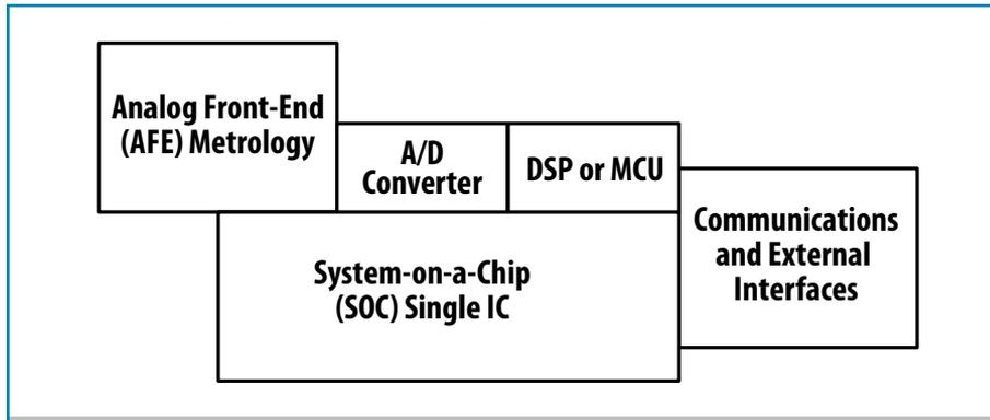
Figure 2B. | Single-Chip Architecture
