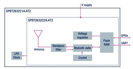
ST's SPBT2632 offers a fully-integrated and fully-qualified Bluetooth solution, ready to use with the smallest footprint available in a simple to handle SMD package.
