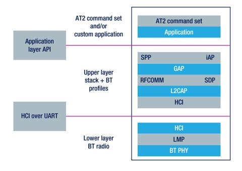
The AT2 command set fully exploits the Bluetooth stack and efficiently supports communication with Androidsmartphone and Apple iOS Bluetoothenabled devices.
